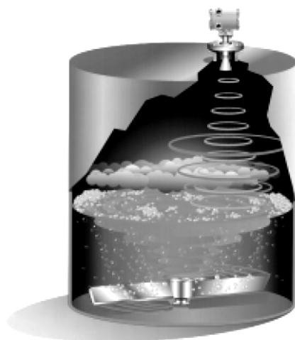
Level Transmitter with RADAR Sensor
