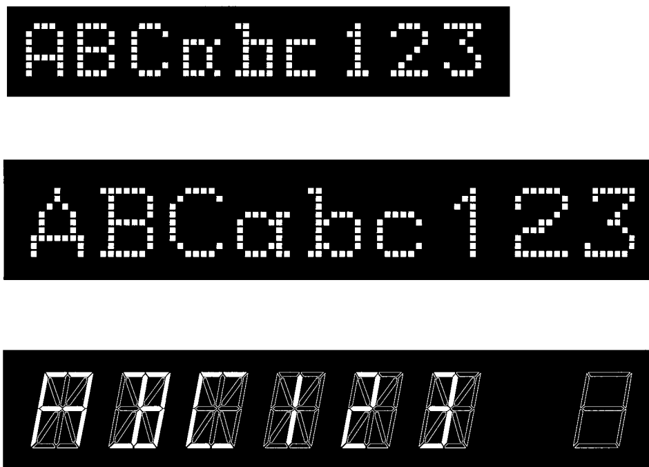
FIGURE 4 Types of alphanumeric matrix displays. (Top) 5 by 7 dot matrix. (Middle) 7 by 9 dot matrix. (Bottom) Bar matrix. (MICRO SWITCH.)
